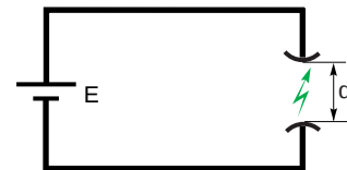
Fig. 2 : electric arc and influence of field E/d value.
